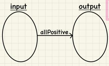
Postcondition checks to see if the output is correct w.r.t. the input.
